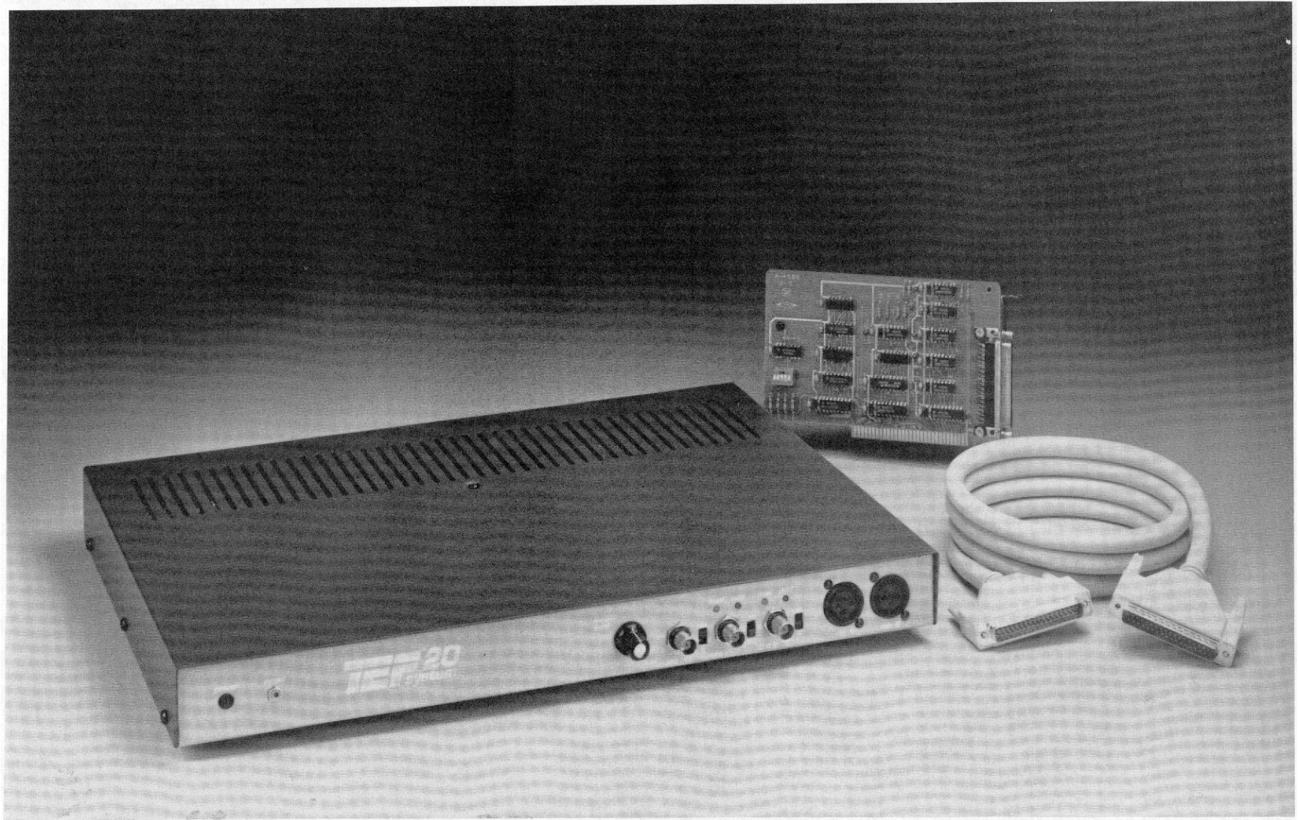
Fig. 1. Photograph of the TEF System 20 HI System. The test analyzer includes a 17-in. x 12 \frac{3}{8} -in. x 1 \frac{3}{4} -in. box which contains the DSP, power supply, A/D and D/A, processing circuitry, and input and output circuitry and connectors. Also shown is the supplied IBM PC compatible parallel interface card with interconnect cable. Up to four interface cards can be used in the PC.
